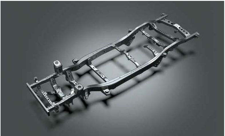
Tough Body on Frame Chassis
