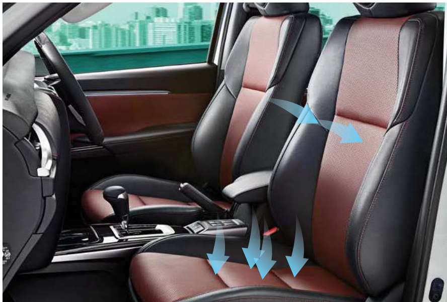
Superior Suction based Seat Ventilation System
