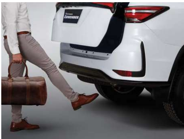
Kick Sensor for Power Back Door
