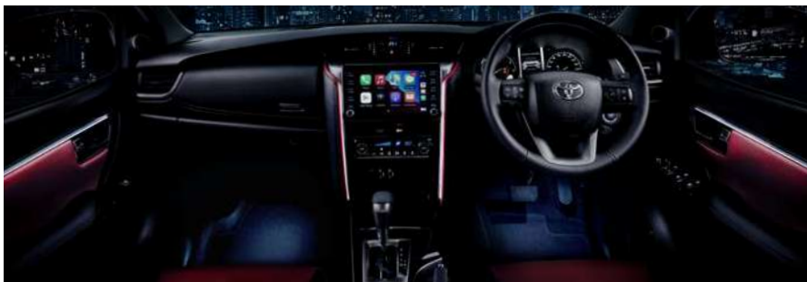
Interior Ambient Illumination for Instrument Panel, Front Door Trim & Front Foot-well Area
